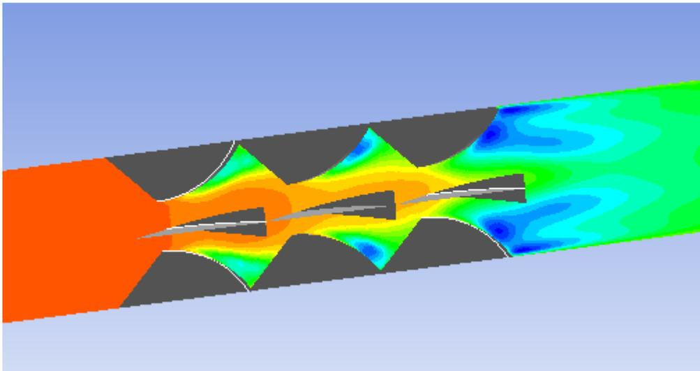
*Figure 3 - Cavitation Pressure in Westfall 3050 Triple Mixer*
