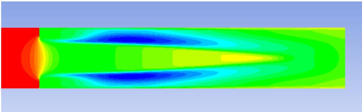
*Figure 1 - Cavitation Pressure Downstream of an Orifice (Beta = 0.67)*
