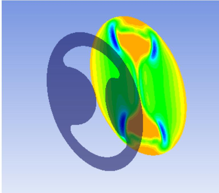
*Figure 2 - Cavitation Pressure 0.4D Downstream of a 2800 0.8 Beta Mixer*
