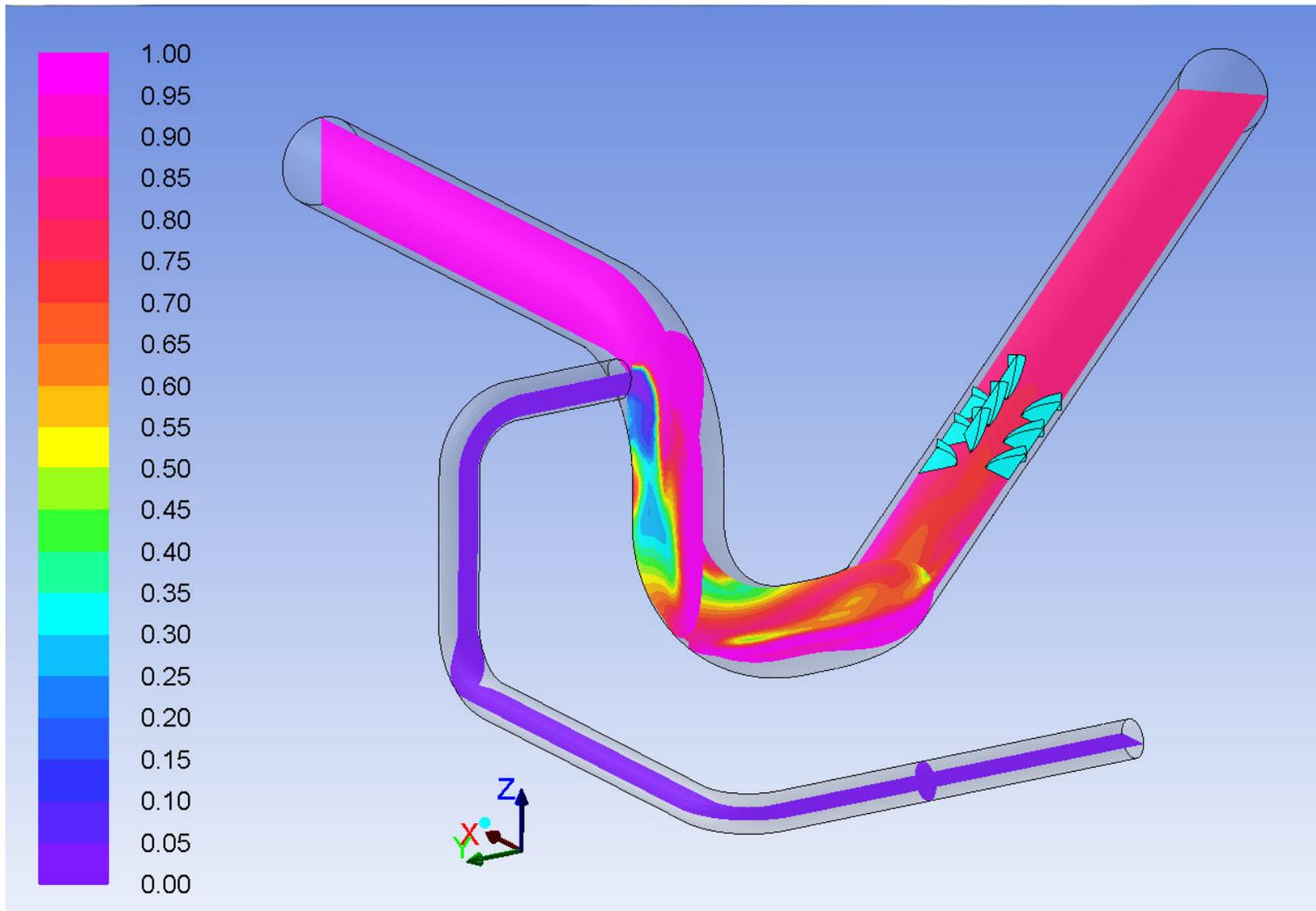
Figure 6 - Contours of Mass Fraction of Perchlorate Solution from Agate Reservoir (High Water Level).
