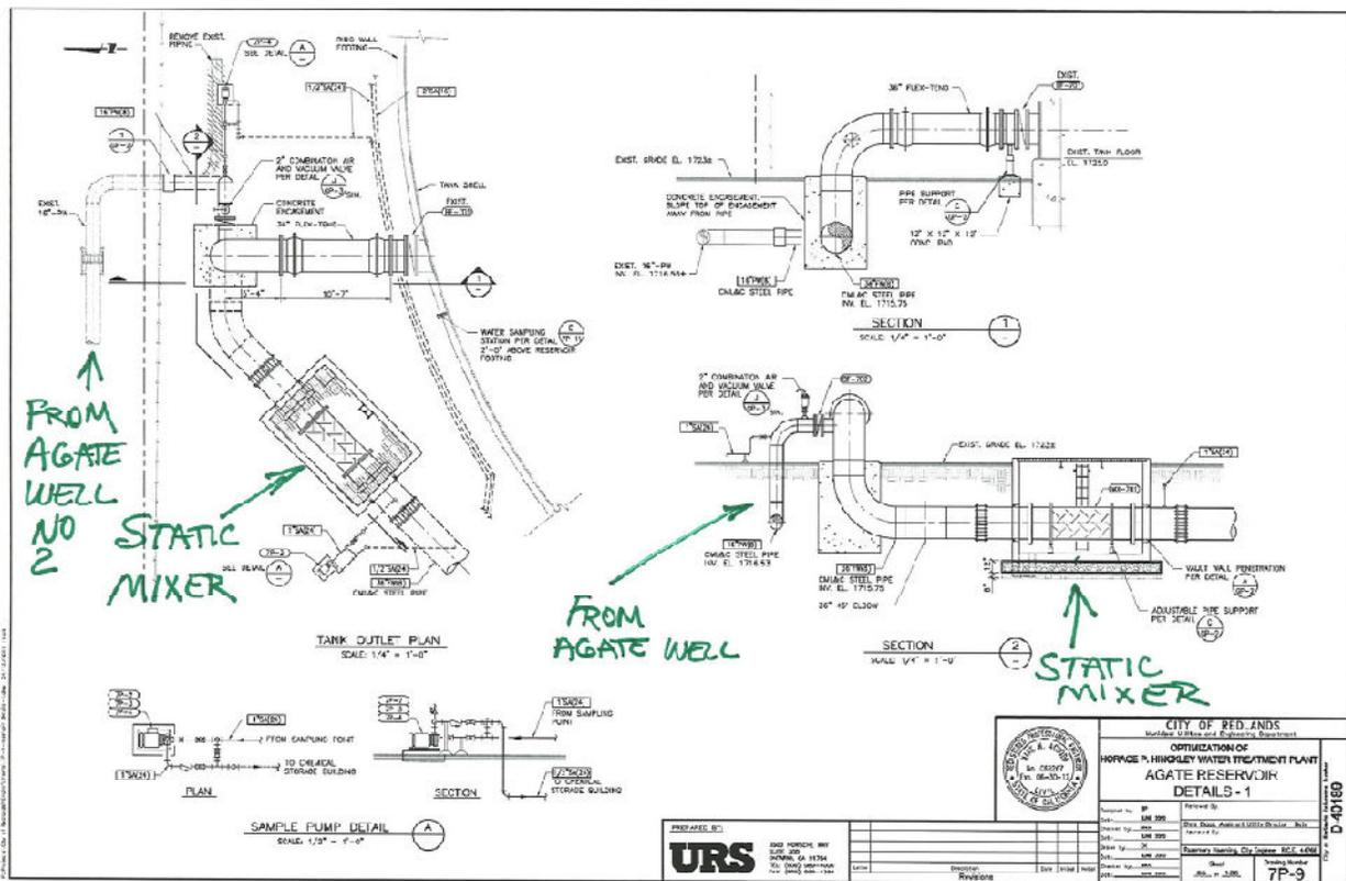
Figure 1 - Static Mixer Piping Layout
