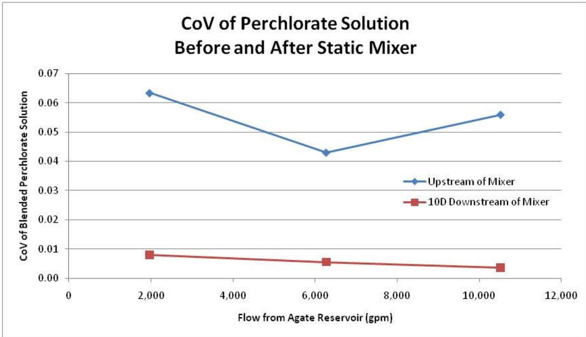
Figure 3 - CoV of Perchlorate Solution Before and After Static Mixer
