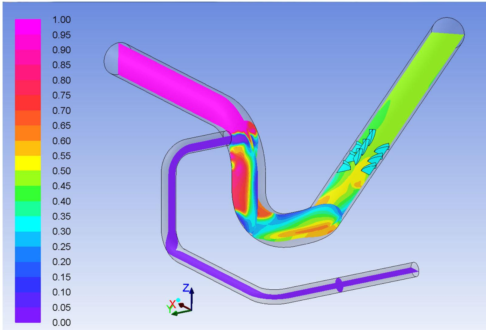
Figure 4 - Contours of Mass Fraction of Perchlorate Solution from Agate Reservoir (Low Water Level).
