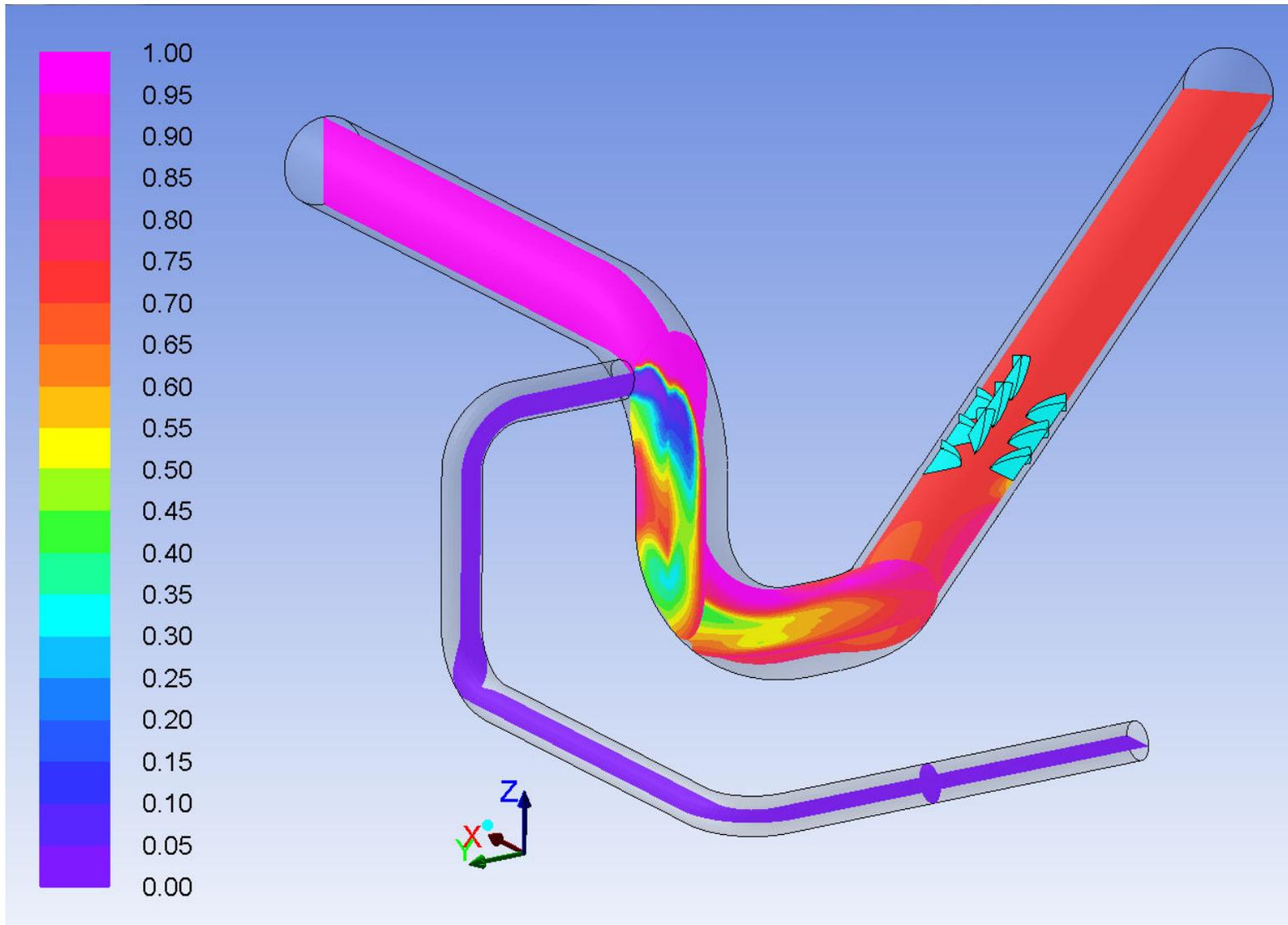
*Figure 5 - Contours of Mass Fraction of Perchlorate Solution from Agate Reservoir (Medium Water Level).*
