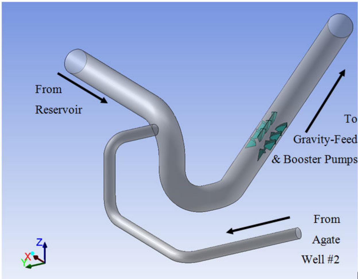
*Figure 2 - CFD Model Domain, Standing at NE, Looking SW*
