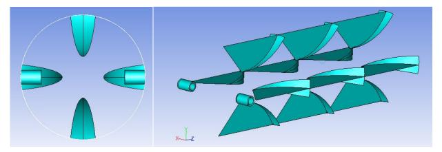
Injection nozzle location with triple mixer configuration.
