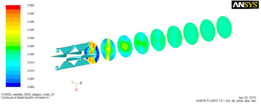
Profiles of concentration downstream of double in line 3050 mixer. Average concentration = 0.02
