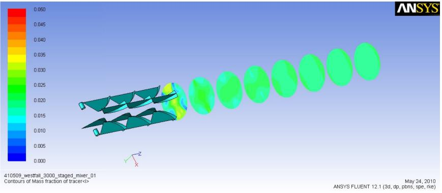
Profiles of concentration downstream of triple in line 3050 mixer. Average concentration = 0.02
