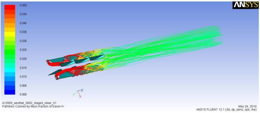
Pathlines from injection ports colored by concentration downstream of triple in line 3050 mixer. Average concentration = 0.02
