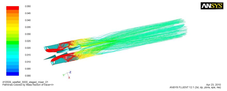
Pathlines from injection ports colored by concentration downstream of double in line 3050 mixer. Average concentration = 0.02
