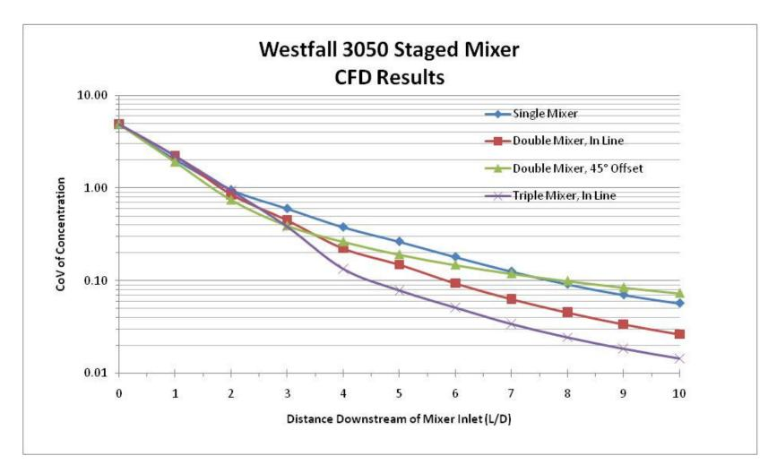
CoV of Concentration in a 6-in ID steel pipe with 2 opposing injection ports, and a mixed tracer concentration of 2%.
