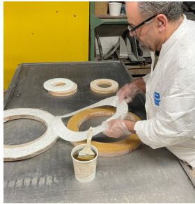
Adding layers of roving to re-enforce mounting ring.
