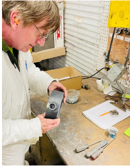
All FRP static mixer - Finishing mixer - installing connectors, inspection and tagging.
