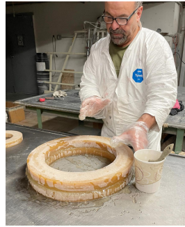
FRP mounting ring lay-up
